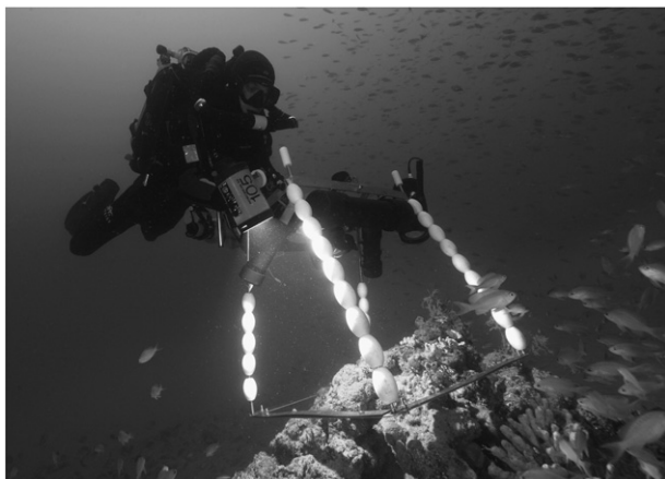
Fig. 3. Photographic quadrat system used in the field. A digital camera was perpendicularly fixed 50 cm over the quadrat frame.
