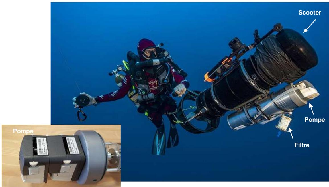
FIGURE 3 : POMPE ETANCHE CONÇUE PAR SUBSPACE, ANDROMEDE OCEANOLOGIE ET L'UNIVERSITE DE MONTPELLIER.
